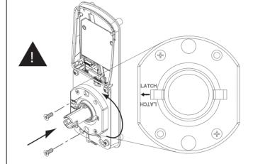
d. Reinstall cover and reader onto baseplate
